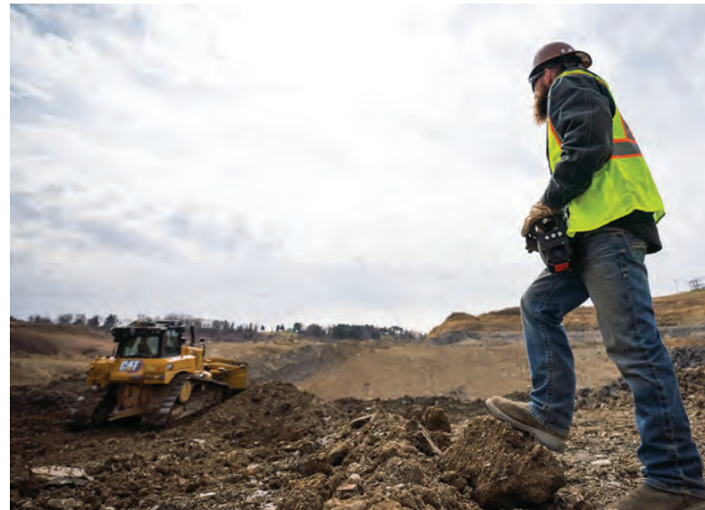
ABOVE AND BELOW: The line-of-sight (LOS) Command Console allows the user to work safely and comfortably away from the machine while remaining onsite and maintaining direct visual contact with the equipment. This option is ideal for short-term and emergency use when encountering potentially hazardous work areas.
