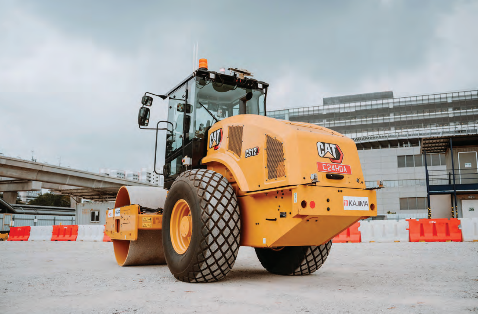
ABOVE BELOW: In the first phase of the project, four autonomous machines – two excavators and two compactors – will be tested at the Bulim Autonomous Yard (BAY), JTC’s sandbox in the Jurong Innovation District. The pilot is targeting a 50% reduction in manpower, with one operator overseeing two machines.
