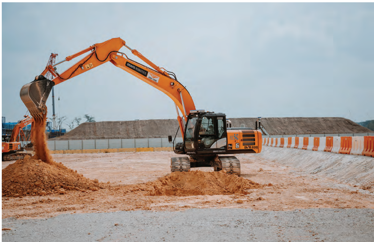
ABOVE BELOW: In the first phase of the project, four autonomous machines – two excavators and two compactors – will be tested at the Bulim Autonomous Yard (BAY), JTC’s sandbox in the Jurong Innovation District. The pilot is targeting a 50% reduction in manpower, with one operator overseeing two machines.
