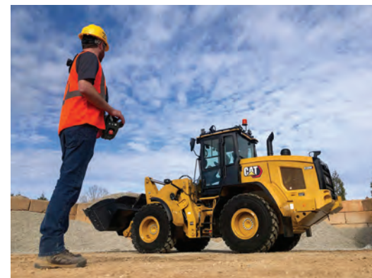
LEFT: Remote-control operation not only enhances safety and productivity but also eliminates exposure to machine vibrations, thus reducing fatigue and allowing operators to work for longer periods.
