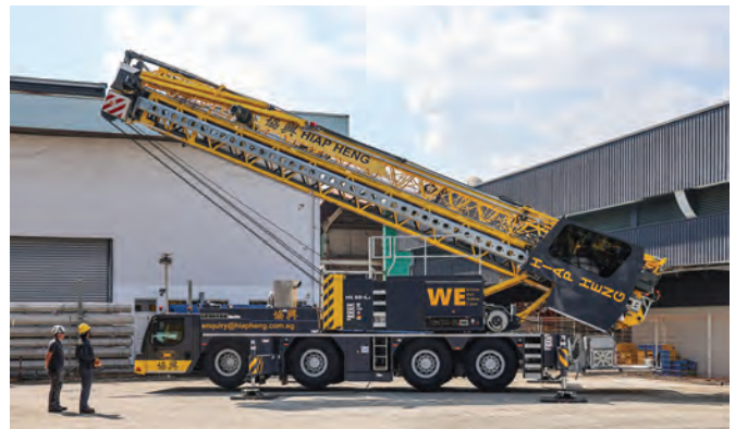
ABOVE: Hiap Heng enters the mobile construction crane segment with the acquisition of its first Liebherr MK 88-4.1E. The crane can be erected quickly and set up by a single person.
