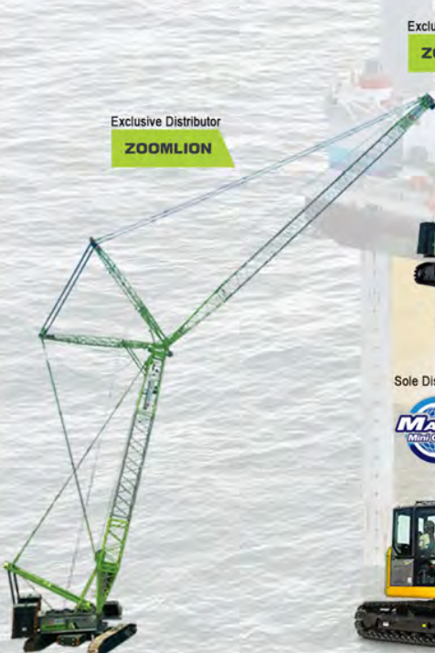
Crawler Crane with luffing jib
