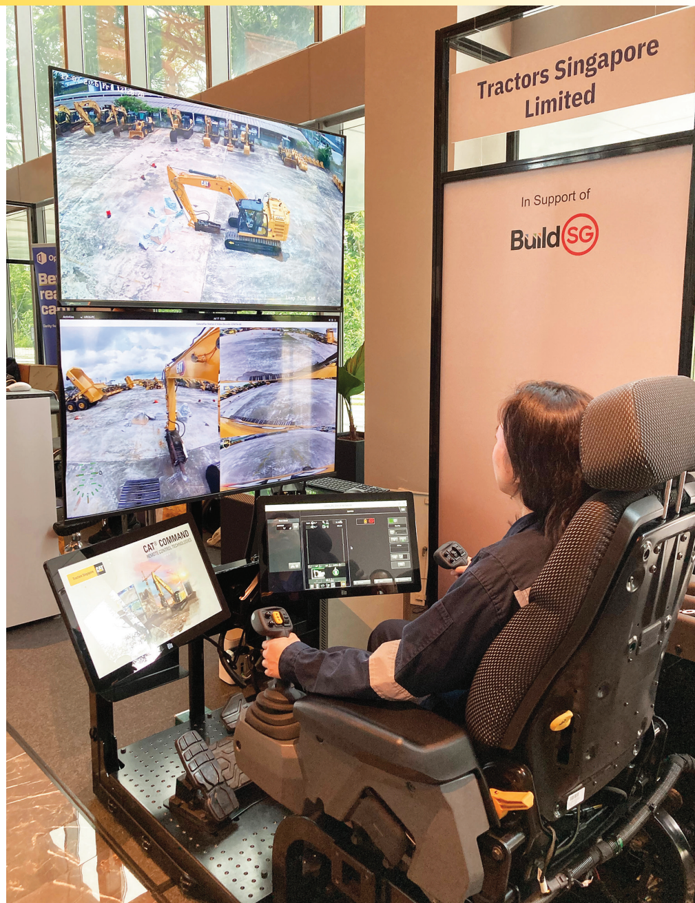
Cat Command remote-control technology is compatible with wheel loaders, dozers and excavators, enabling operators to remotely perform loading, dozing and excavating operations. One of the options, the non-line-of-sight (NLOS) Command Station, includes a modular, customised 'virtual cab' where the user is comfortably seated in front of machine controls and displays similar to those inside the operator's cab.
